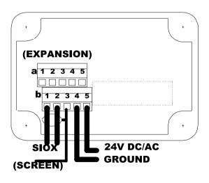
These 4 or 5 communication/supply wires are installed in either of two parallel 5-pole terminal strips in the junction box. The other strip is free for extension wiring to further distributed unit(s).
