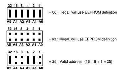
The jumper positions A0 - A5 contribute their values 1, 2, 4, 8, 16 and 32 when the corresponding jumper is <u>removed</u>.
