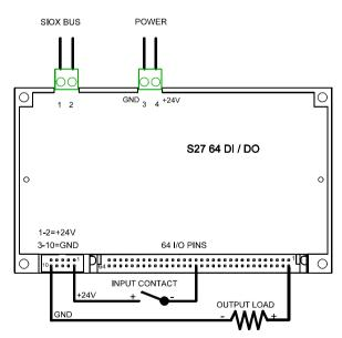
capacitive load on the SIOX bus and decrease the maximum distance over which communication can be carried out for a given bit rate. The total resistance of the bus should not be higher than 2 \* 50  $\Omega$ .
