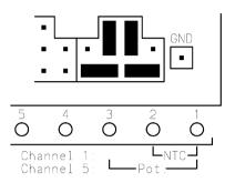
The same two jumpers as in 10 V modes are installed to decrease the input signal, one for either channel. In addition, an extra jumper for each channel connects the current source to the input pins. Connection is independent of the sensor type.
