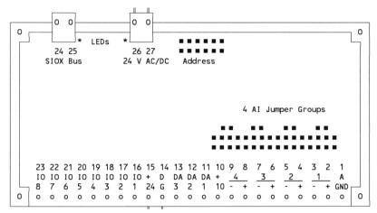
The power supply can be any AC or DC voltage of 12 - 35 VDC or 15 - 24 VAC. The module itself consumes less than 20 mA, but the digital outputs can output above 2 A together. For high-current loads it is therefore recommended to use a DC supply and connect it, correctly polarized, to terminals 14 and 15 of the 23-pole I/O-connector. This bypasses the 400 mA rectifier at terminals 26 and 27 and limits rectification ripple.
