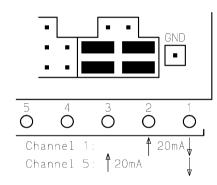
In addition to the jumpers that divide the differential signal before measurement, another two connect current measurement resistors from the input pins to ground. For maximum flexibility, either half of the terminal pair may be modified to suit another single-end input mode.
