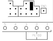
Only one jumper is installed between the top and middle rows to supply the transducer current. In Pt100 Mode full sensitivity is needed and both jumpers in the bottom row shall be removed. Note that full amplification makes the inputs more sensitive to overvoltages. Although the inputs are well protected, adjacent channel measurements may be affected, so install these jumpers on all unused channels.
