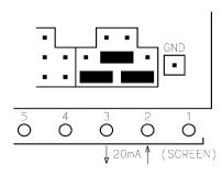
In addition to the jumpers that divide the differential inputs before measurement, another jumper connects a current measurement resistor between the input pins. In addition to the signal wires to terminals 2 and 3, any cable screen or signal grounding point for the input signal is best connected to terminal 1, Analogue Ground.
