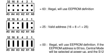
The jumper positions A0 - A5 contribute their values 1, 2, 4, 8, 16 and 32 when the corresponding jumper is removed.
